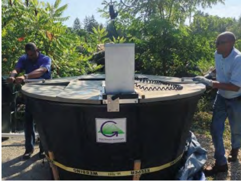
Recycling Operations Manager Barry Wilkins and Recycling Technician Leslie Gibson turn the lid of the "Earth Tub" composting unit. The tub composts most of the food preparation waste collected from campus kitchens.
